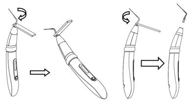
Tighten clockwise to install the tip
